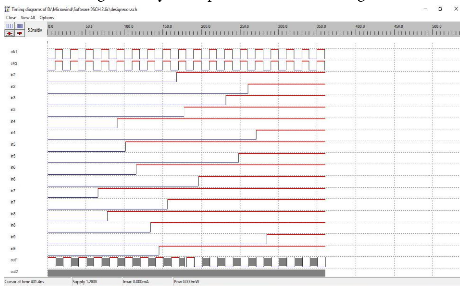
Figure 3 Timing Representation of Dynamic EX-OR gate
